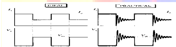
Figure5: Typical switching waveforms of (a) hard-switched and (b) soft-switched devices
